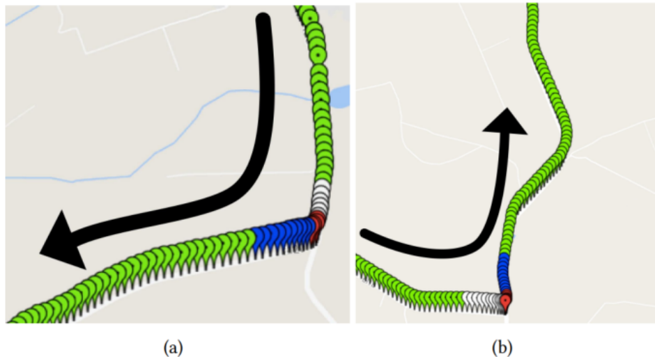
Figure 5: Two real-world turns in the driving session. The pin color represents cluster assignment from our TICC algorithm (Green = Going Straight, White = Slowing Down, Red = Turning, Blue = Speeding up). Since we cluster based on structure, rather than distance, both a left and a right turn look very similar under the TICC clustering scheme.
